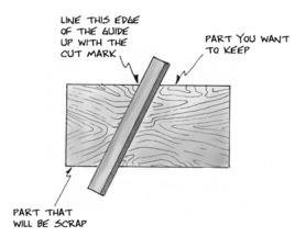
The guide must be firmly secured to the work. You can do this by clamping it down or by using drywall screws. The clamps are sometimes problematic when the saw motor doesn't have enough clearance to move over the tops of the clamps but the screws leave holes.
