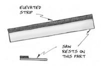
USE TWO STRIPS OF PLYWOOD TO MAKE A CIRCULAR SAW GUIDE
